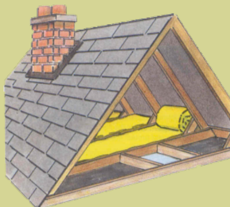
Figure 4: Thermal insulation of a roof may be very easy to apply.
